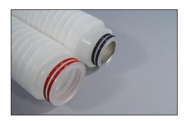
PNM Membrane Filter Cartridges are sterilizing grade nylon cartridges. The nylon membrane used in these cartridges is optimized for retention. Nylon cartridges see broad service in sterile fill applications in SVPs and as bioburden management filters in LVPs. Media and service liquid filtration are other common applications for this cartridge. Nylon is particularly suited for the filtration of solvents because of its broad compatibility and low level of extractables.
